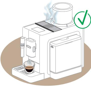
**EN** Tilt the tank to enable its removal
